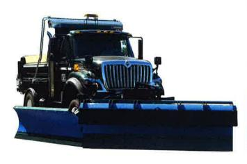
Full hydraulic lift, rigid or trip cutting edge design. Hydraulic teletube option for maximum visibility through passenger door window, for left or right hand mounting.
